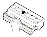
**11.** Replace the toner cartridge. Hold the handle of the toner cartridge so that the stamped markings on top of the cartridge are facing upward.
